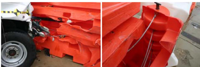
Four Cables Preventing Vehicle Breaching
