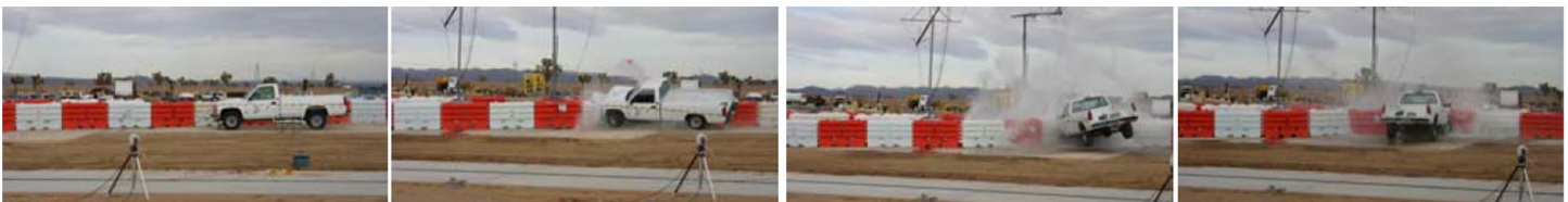
Four Cables Preventing Vehicle Breaching
