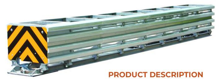
The Smart Cushion® crash attenuator is a revolutionary, speed-dependent product that varies stopping resistance during an impact. The SCI 100 GM Attenuator crash attenuator allows lighter and slower-moving vehicles to have longer ridedown distances and lower ridedown g-forces.
