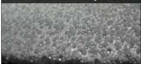
Material after heating with ideal 60% glass bead embedment for optimal performance
