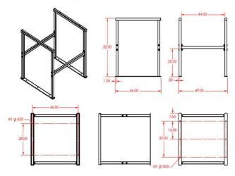
**BED MOUNT FRAME**Mounted directly to vehicle bed.
