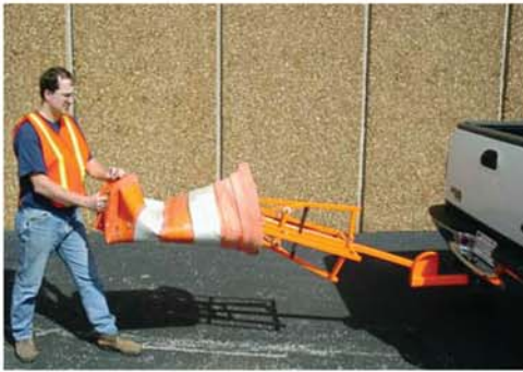
Place damaged drum over Drum Dr.
